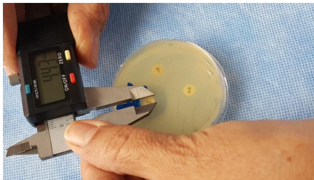
Figure. 5: Shows the digital meter ruler that used for measure the inhibition zones
